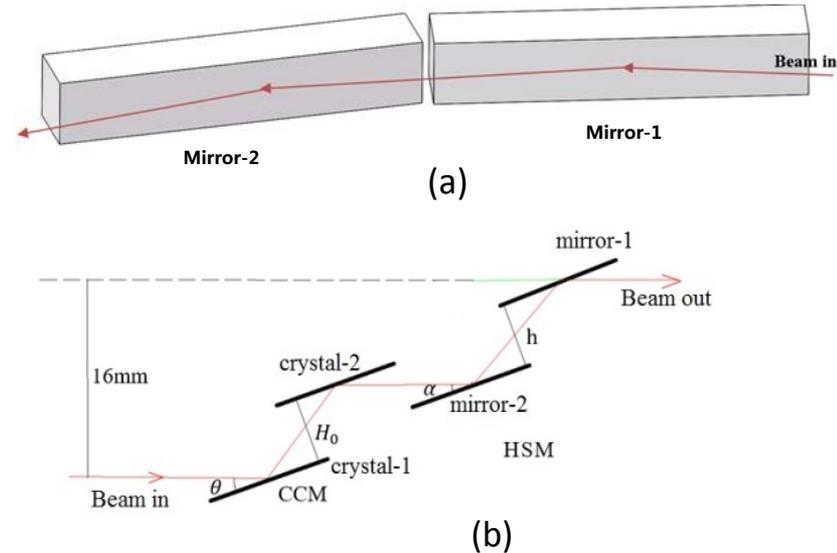
Figure 9: Principle diagram of the double mirrors system. (a) CDM. (b) Complicated HSM for the height compensation of the channel cut mono. (CCM) at B8-XAS beamline.
