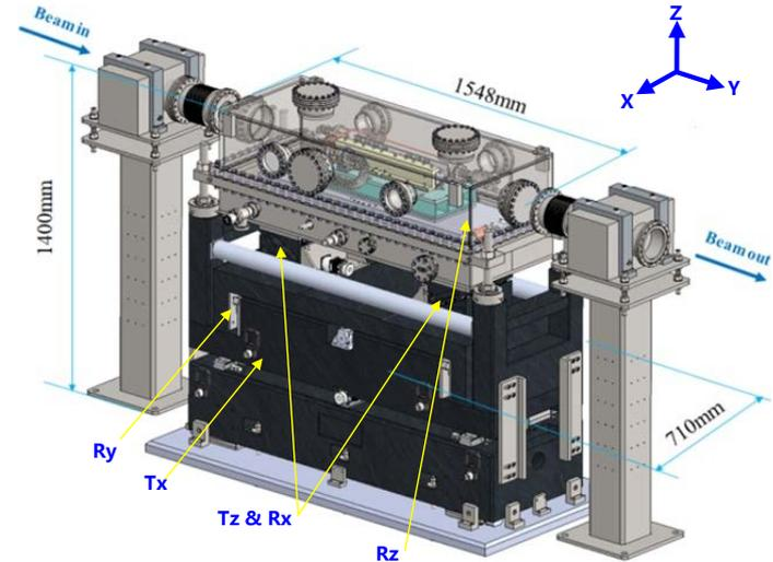
Figure 4: The overview of the typical design of GMMS.
