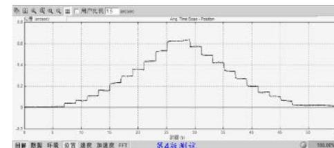
0.25 $\mu\text{rad}$  angular step test results
