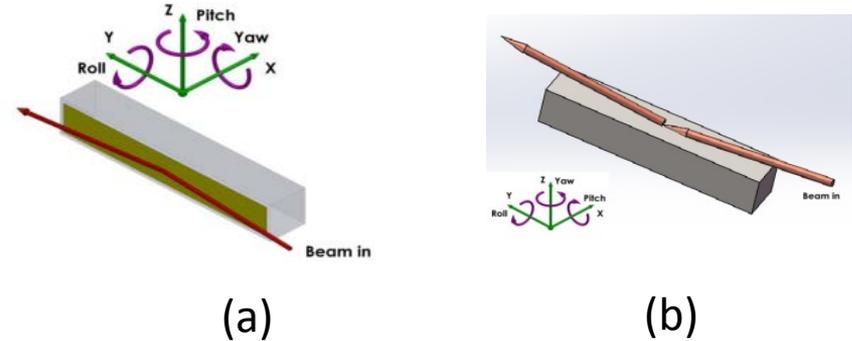
Figure 3: Layouts of horizontal and vertical reflection mirrors. (a) Horizontal reflection. (b) Vertical reflection.
