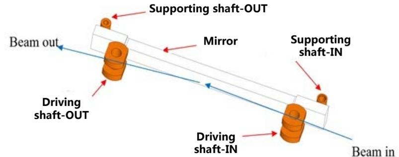
Figure 7: Principle diagram of an independent four-shaft bending
