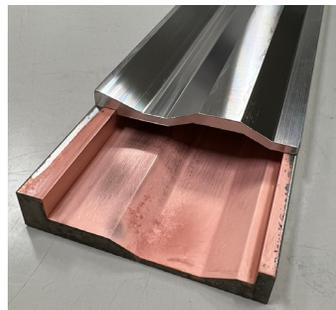
*SUS316L chamber and copper plating is not continuously developed.*
