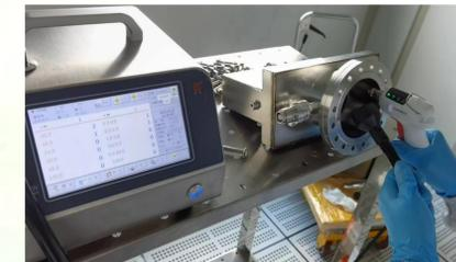
The valves used in SHINE beamline vacuum is all-metal, therefore, valve open/close action always generate particles. Tests have been carried out for angle valves and gate valves, the results show that every single open/close action could generate dozens of particles at 0.3 and 0.5 um size.
