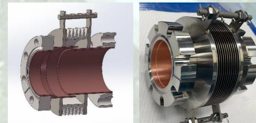
To avoid friction between metals which could generate the large number of particles, a non-contact type RF shielding bellow design is adopted in room temperature beamline vacuum. This RF bellow has 2 copper tube nested inside and out, with a radial direction offset 2 mm.
