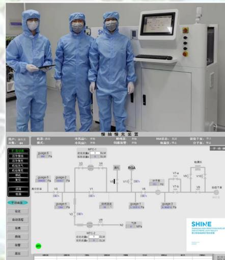
Several kinds of full-automatic slow pumping & slow venting (SPSV) systems have been developed for particle-free vacuum system. The mass flow rate in pumping and venting procedures could be set down to 0.2 SLM, so as to avoid turbulent flow and reduce the probability of contamination and particulates transporting in vacuum system.
