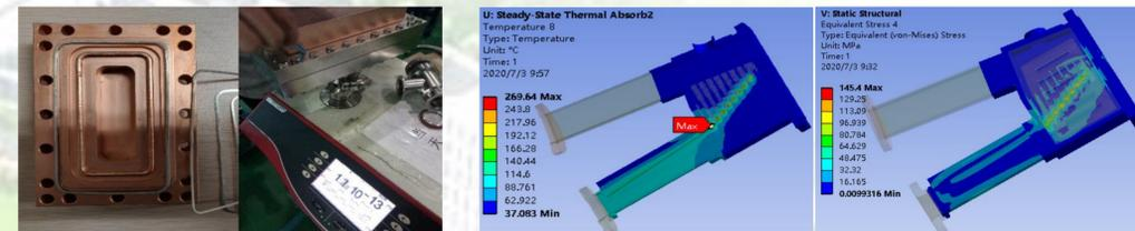
Several welding process were carried out to complete photon absorber 2 fabrication because of complex structure. Friction welding was mainly adopted for absorbers fabrication to keep the temperature of absorbing face bellow 500 °C, avoiding deterioration of material properties.
