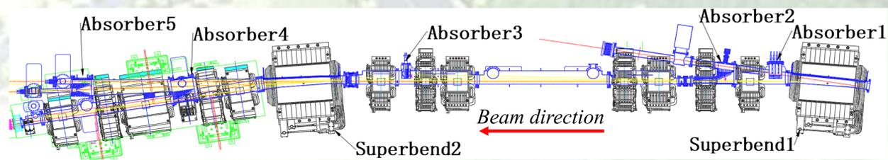
All absorbers were installed at clearance of each couple of magnets. Ion pumps were installed next to these absorbers to enhance pumping efficiency. The maximum heat flux density on absorber 2 is yet up to 43W/mm<sup>2</sup> @300mA after structure optimization.
