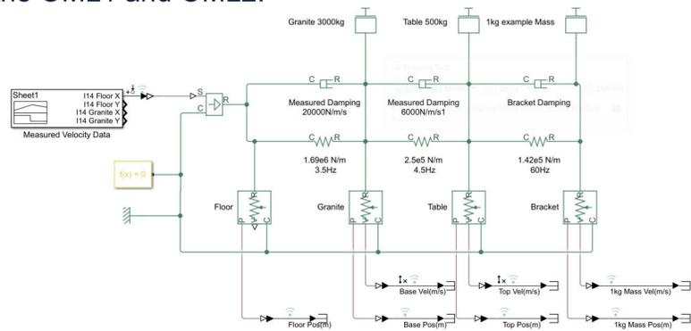
Simulink lump mass model of 2 DOF system.
