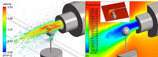
Temperature and velocity distribution around the sample
