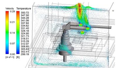
Distribution of the velocity vectors towards the upper zone, due to the thermal load of the three cameras
