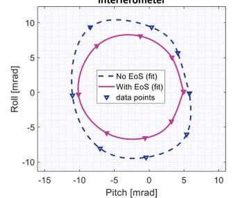
Replacement of C01 interferometer to the F04 model from SmaAct extended the reading range to the full 15 mrad of operation, also enable an End of Stroke (EoS) self-test.
