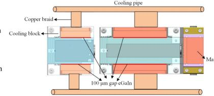
Fig. 3: The mechanical structure of the cooling part.
