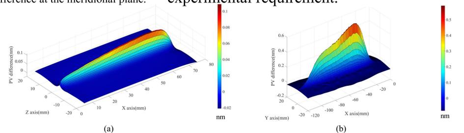
Fig. 5: The thermal deformation PV difference on the mirror surface of HKB (a) and VKB (b).
