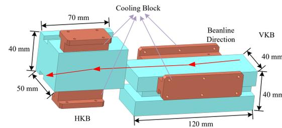
Fig. 2: The distribution of Cu cooling block of HKB and VKB.
