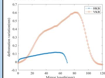
Fig. 6: The thermal deformation PV difference at the meridional plane.
