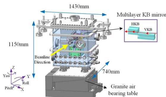
Fig. 1: The mechanical structure. (a) The external overview. (b) The multilayer KB mirror system.
