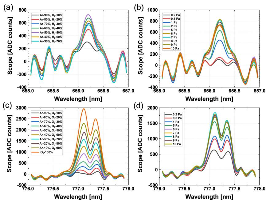
In Ar/O<sub>2</sub> plasma cleaning, although 100% oxygen produces more reactive oxygen species, the total number of ions in the chamber will be less, as shown in the figure below. Considering the physical sputtering effect during cleaning, the Ar/O<sub>2</sub> plasma cleaning ratio will be adjusted to 30%-70%.
