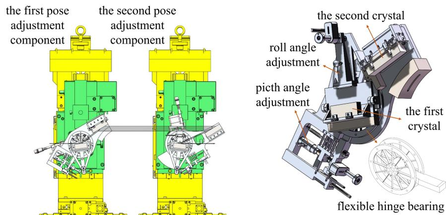
Figure 1: Mechanical design of the HRM.
