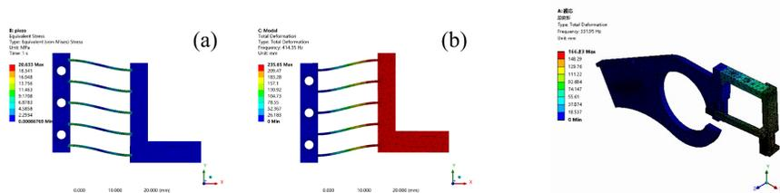
Figure 4: FEA of the flexible guide mechanism. (a) Stress:21 MPa and (b) modal:414 Hz.
