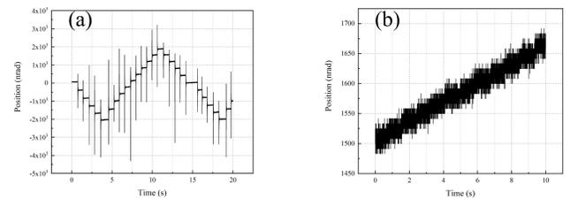
Figure 9: Resolution test. (a) Coarse adjustment resolution:250 nrad and (b) fine adjustment resolution:8.3 nrad.
