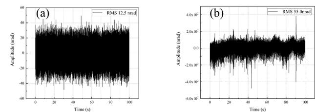
Figure 10: Stability test. (a) The stability between the first and second crystals:12.5 nrad RMS (0.5-500Hz) and (b) the stability between the first and second mechanisms:55.0 nrad RMS (0.5-500Hz).
