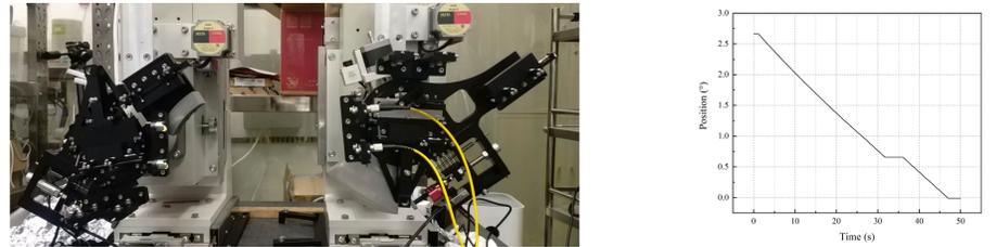
Figure 7: Experimental device. Figure 8: Stroke test of coarse pitch:  $\pm 1.3^\circ$ .
