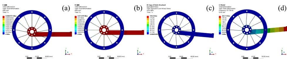
Figure 3: FEA of the flexible hinge bearing. (a) Radial stiffness:26802 N/mm, (b) axial stiffness:886 N/mm, (c) stress:196 MPa and (d) modal:58 Hz.
