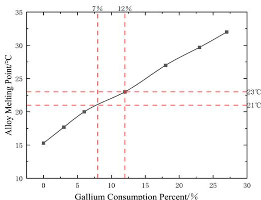
FIG. 2. Melting point curve of the alloy.
