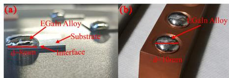
FIG. 3. Sample with EGaIn alloy. (a) substrate sample (b) coating sample
