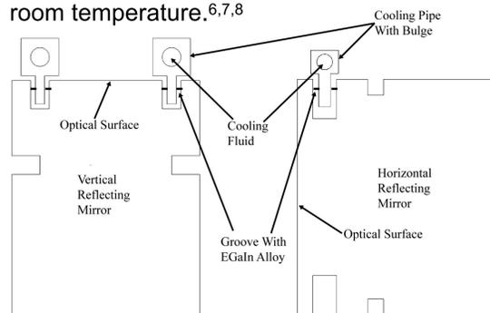
FIG. 1. Vibration decoupling cooling.
