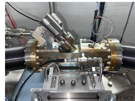
Installed CuCrZr thermal-cycling test body
