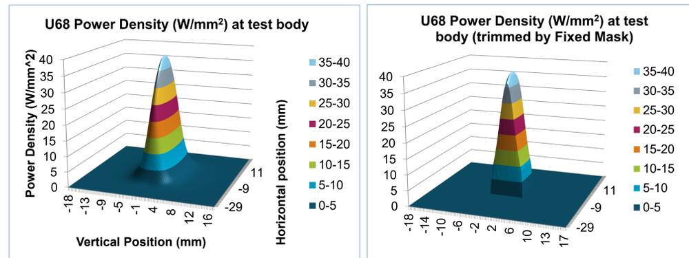
U68 power density (~16 kW/mrad<sup>2</sup>) is smaller than the nominal power density for a typical front end (100 kW/mrad<sup>2</sup>). Total Power = ~5.2 kW @ 500 mA
