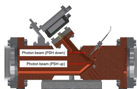
CuCrZr thermal-cycling test body
