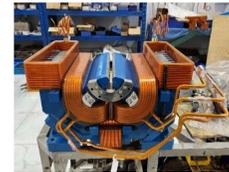
pre-installed dowel; remove upper half yoke; install correction coils.
