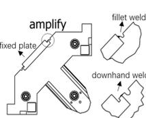
Downhand welding & robot welding to reduce distortion.
