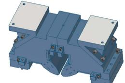
Confirm mounting hole positions when milling the bottom surface.
