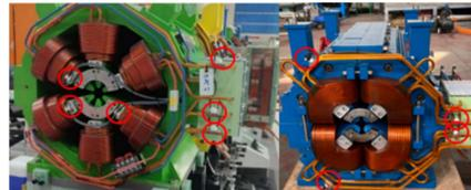
Switch distribution close to the pole: sextupole ( $36 \pm 3^\circ\text{C}$ ); quadrupole ( $43 \pm 3^\circ\text{C}$ )
