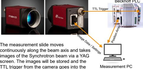
The measurement slide moves continuously along the beam axis and takes images of the Synchrotron beam via a YAG screen. The images will be stored and the TTL trigger from the camera goes into the PLC. The PLC will store the position at the moment where the trigger signal comes in. This array of the positions can be read immediately after the scan. This is faster than just read the position during the scan over our used Tango Control system.
