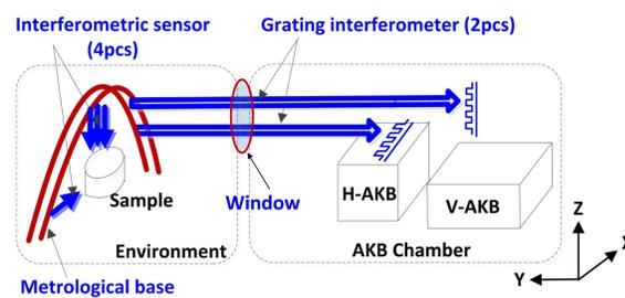
Fig.2 Metrology scheme of proposal method for Hard X-ray Coherent Scattering Beamline (HXCS) at HEP
