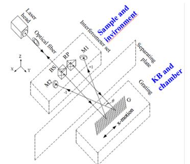
Fig.3 Principle configuration of the direct measurement
