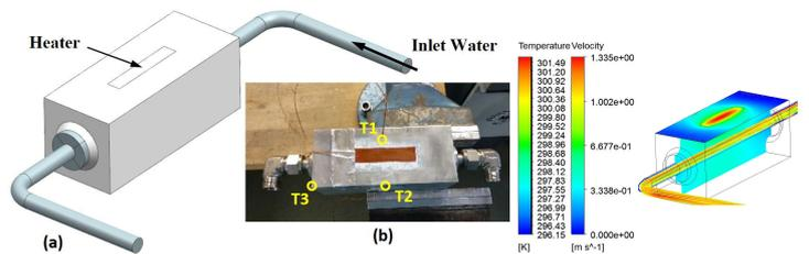
(a) Mirror simplified model, (b) Details of temperature sensors and heater for experiment. Right: Velocity and temperature distributions for the case CFD  $k - \omega$  SST, 43.4 W, and 1 m/s inlet
