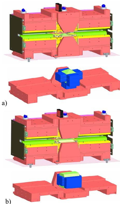
Figure 2: a) 3 T superbend dipole b) 1.2 T standard dipole.
