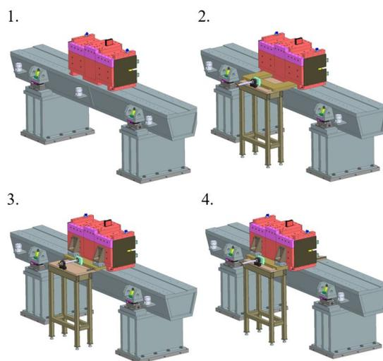
Figure 7: Extracting procedure for dipoles.
