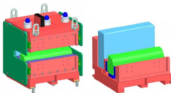
Figure 1: Short dipole 3D model.
