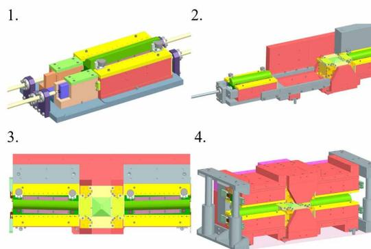
Figure 6: Assembling procedure for long dipoles.
