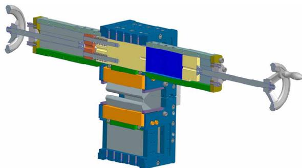
Figure 5: Inserting quadrupole N01 magnets tool.
