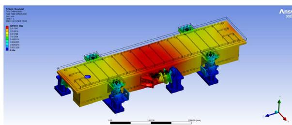
Figure 3: Deformation analysis of the girder system.
