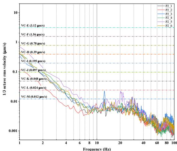
Figure 2: Comparison of the ground vibration and VC.
