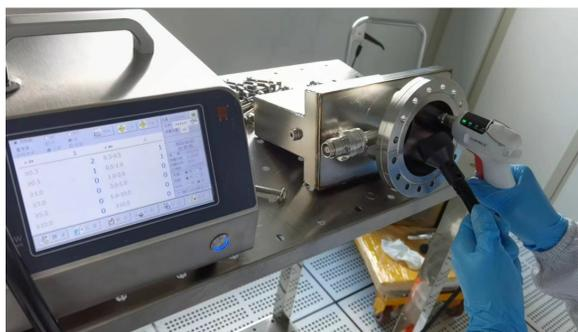
Figure 4: Ion pump assembled in ISO 4 clean room.
