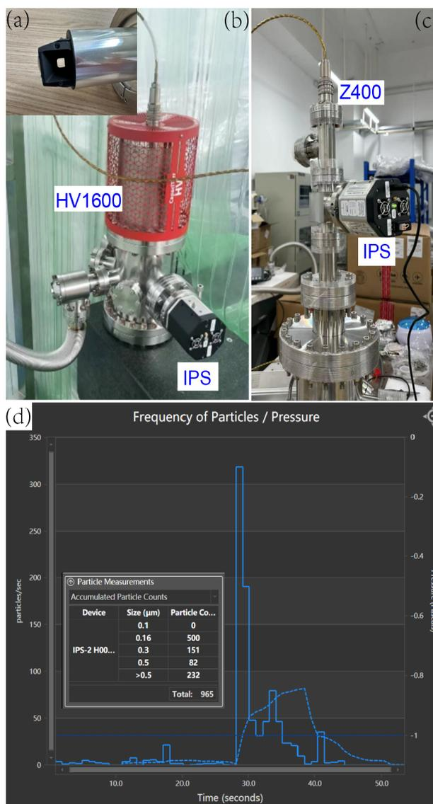
Figure 5: (a) In-vacuum sensor of IPS, (b) Saes HV 1600 getter pump particle test, (c) Saes Z400 getter pump particle test, (d) particle count of IPS.
