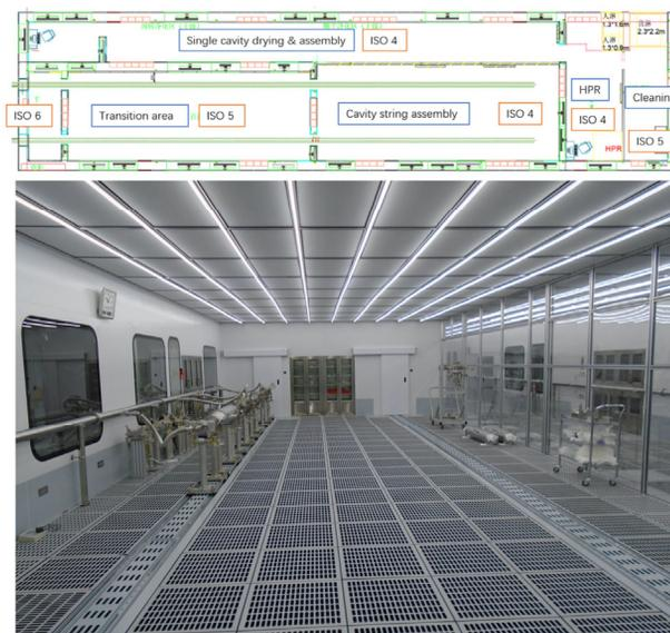
Figure 1: ISO 4 class cleanroom for cavity string assembly.
