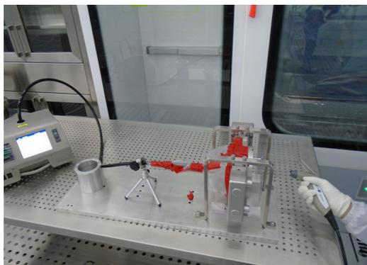
Figure 6: Particle test of valve open/close action.
