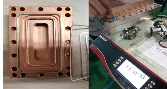
Figure 4: The sample of CuCrZr step flange and seal test.
