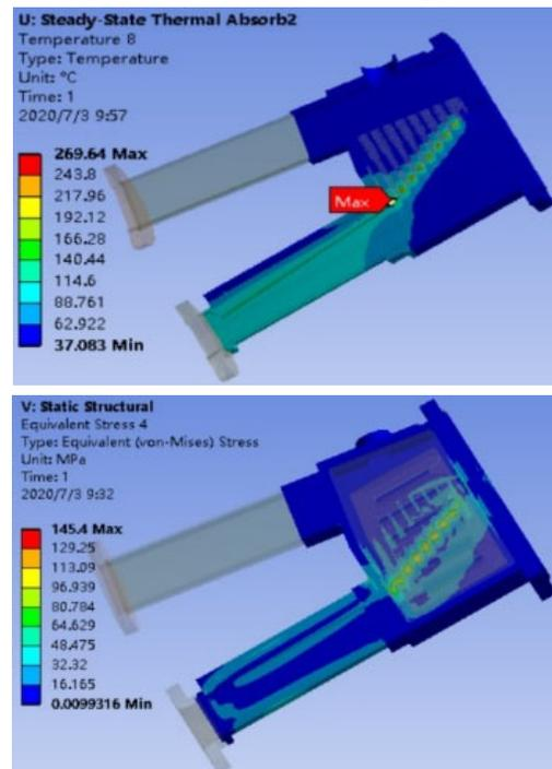
Figure 5: Nephogram of temperature and equivalent stress of absorber 2.
