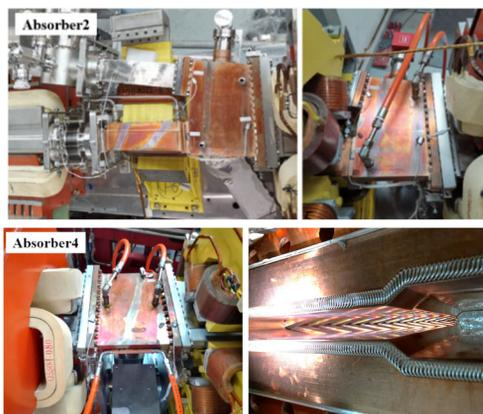
Figure 7: CuCrZr absorbers installed on the storage ring.
