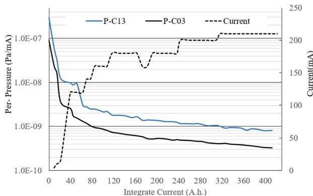
Figure 8: Curves of per-pressure versus integrate current in the early stage of startup.
