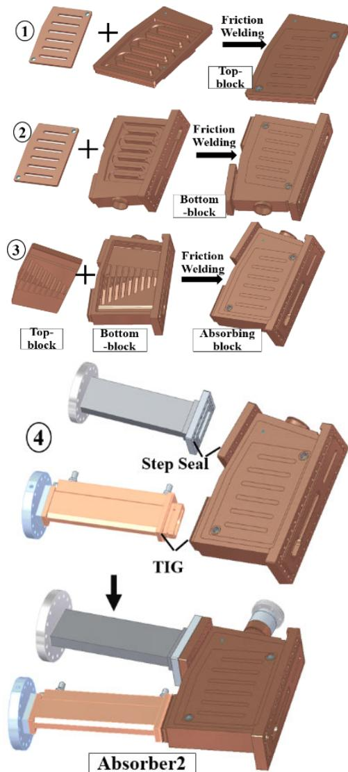
Figure 6: Main fabrication process for absorber 2.
