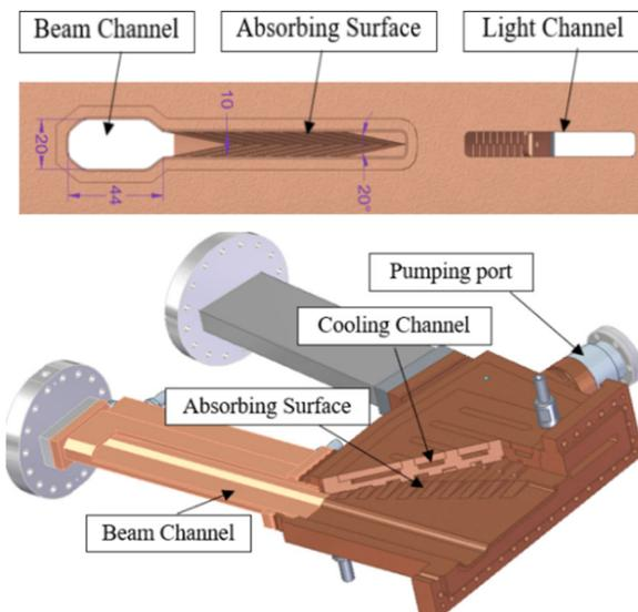
Figure 3: 3D model of the structure of absorber 2.
