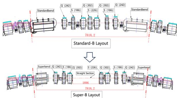
Figure 1: Standard-B section upgrade to super-B section in SSRF.
