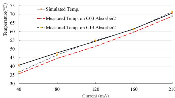
Figure 9: Temperature comparison between simulation and measurement on absorber 2.
