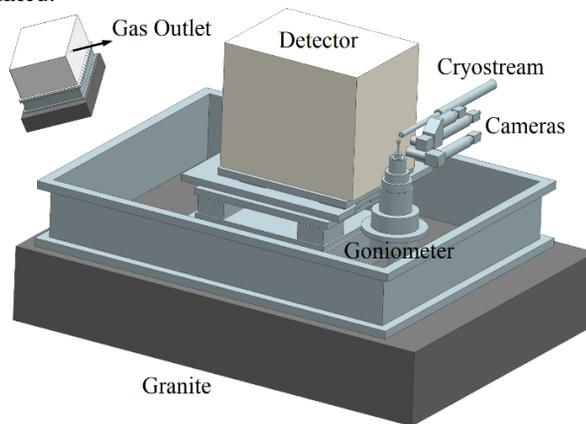
Figure 2: Simplified model of the chamber, showing some of its internal components.
