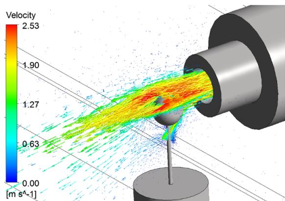
Figure 4: Velocity vectors around the sample.
