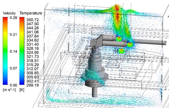
Figure 5: Distribution of the velocity vectors towards the upper zone, due to the thermal load of the three cameras.
