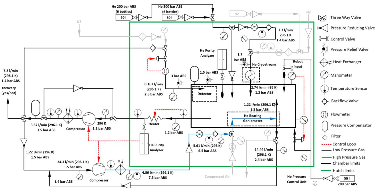
Figure 1: XAIRA PID operational mode 1: Helium gas with Cryostream on.
