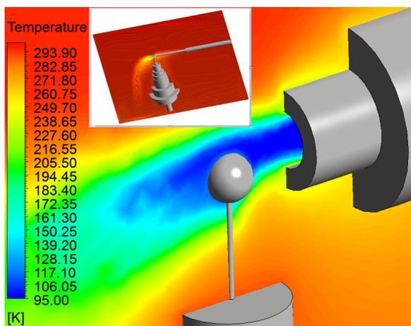
Figure 3: Temperature distribution around the sample and in a vertical plane at the position of the sample.
