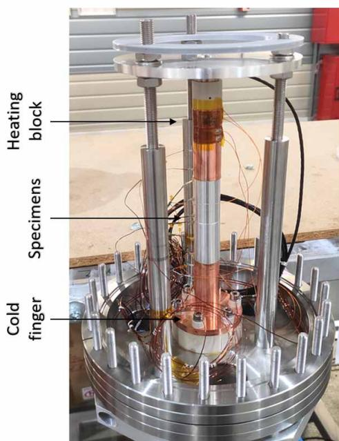
Figure 2: Image of the experimental setup manufactured in ALBA. Note that the specimens are made of aluminium instead of copper for our upcoming tests.
