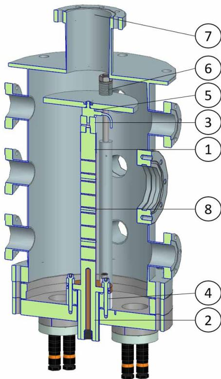
Figure 1: Cross section of the experimental set-up for the evaluation of TCC.
