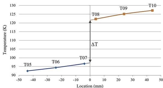
Figure 4: Plot of the temperature at different axial location in both specimens, pressure 0.4 bar.
