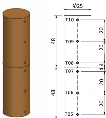
Figure 3: Isometric and front view of the specimens with the location of the temperature sensors.
