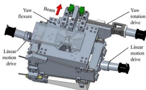
Figure 4: Design of the yaw rotary stage.
