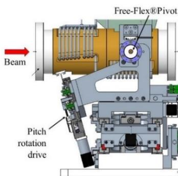
Figure 3: Design of the pitch rotary stage.
