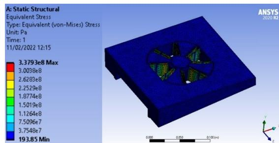
Figure 7: Stress distribution in the flexure.
