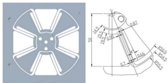
Figure 6: Details of yaw rotary flexure.
