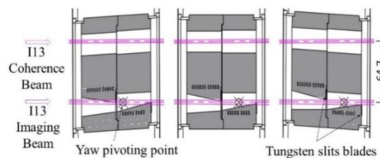
Figure 2: Anamorphic view of sections in X-Z plane showing yaw rotations of the slits. Left: closed position; Middle: neutral position; Right: open position.
