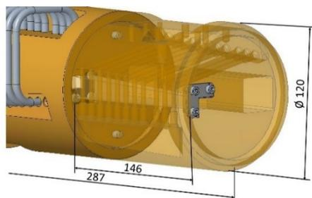
Figure 8: Slit block (downstream cooling pipe hidden).
