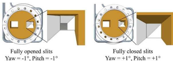
Figure 5: Details of fully opened and closed slits.
