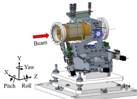
Figure 1: Slit assembly and the coordinate systems.
