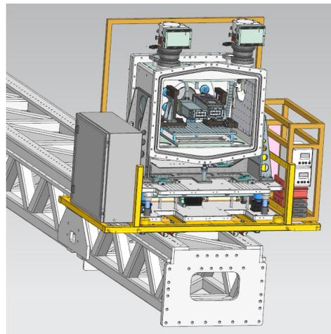
Figure 1: Vacuum chamber with detectors and platform with electronics of the MDS on the arm of the AGIPD at the MID instrument (CAD model).
