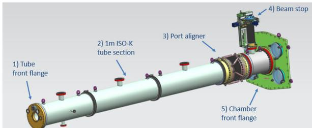
Figure 10: 1) Tube front flange, 2) Flight tubes, 3) port aligner, 4) beam stop, and 5) front flange.
