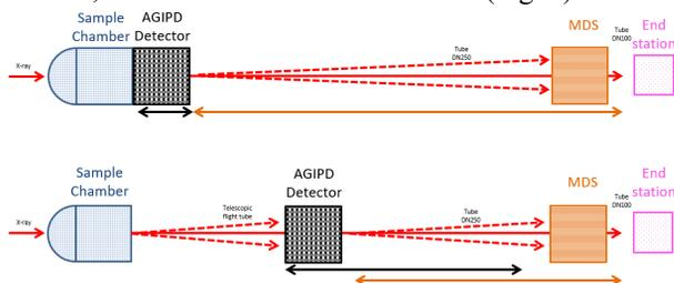
Figure 3: Sketch of the geometry with MDS positioned behind AGIPD on a common detector arm.
