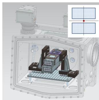
Figure 6: Square setup of two Jungfrau detectors.
