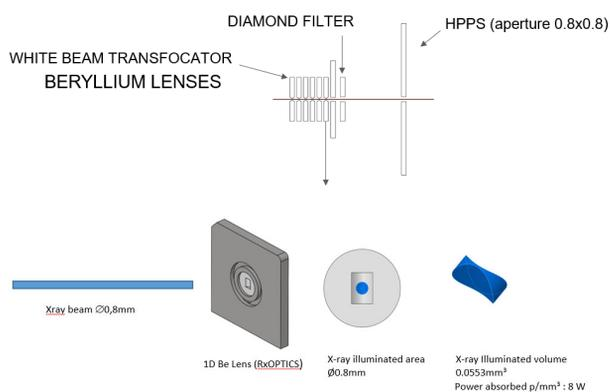
Figure 5: Power absorption at ID14 – Be lens =  $8 \times 0.0553 = 0.45$  W.
