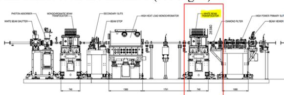
Figure 1: The white beam translocator is installed in OH1 at 28.5 m from source.
