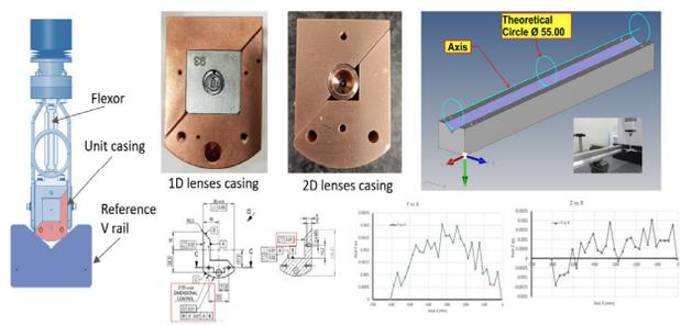
Figure 8: Manufacturing accuracy of 1D/2D casings and reference V rail.
