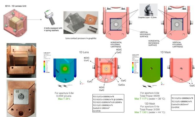
Figure 7: Lenses unit cooling optimization with spacer and thermal interfaces.
