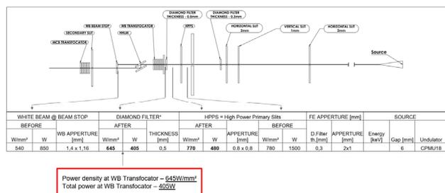
Figure 4: Front End and optical hutch heat loads configuration.
