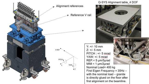
Figure 9: Alignment specifications for WBT (Reference V rail alignment/lenses units) with X-ray.
