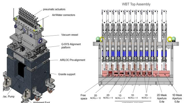
Figure 3: 11 axis water cooled translocator.
