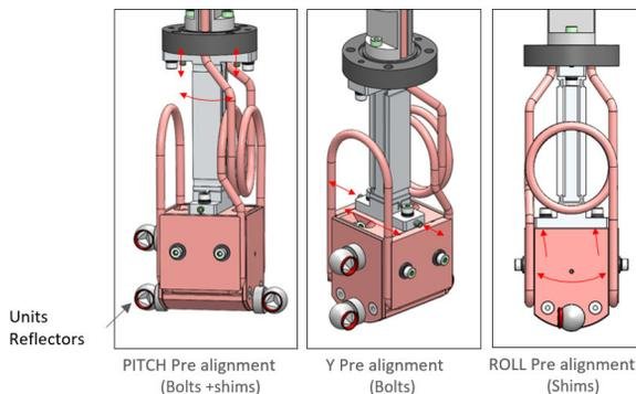
Figure 10: Pre-alignment to limit flexor strokes.
