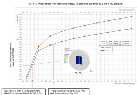
Figure 6: Thermal stress before/after 0.5 mm thick diamond window.
