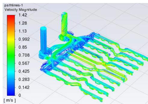
Figure 6: CFD simulation of detector cooling component using ANSYS Fluent.
