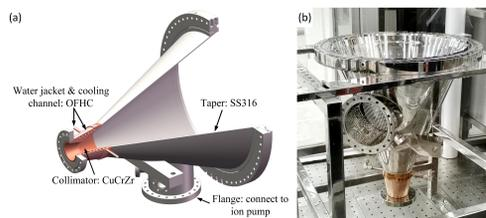
Figure 5: (a) Model and (b) fabricated collimating taper transition.
