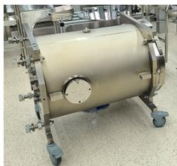
Figure 2: The jacketed 166.6 MHz srf cavity.
