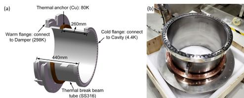
Figure 3: (a) Model and (b) fabricated thermal break beam tube.
