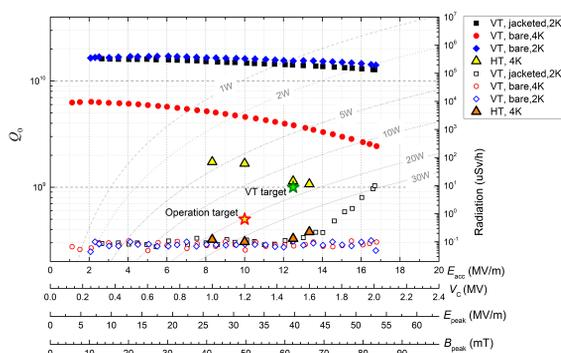
Figure 7: Quality factor and radiation level of the jacketed cavity during horizontal tests.
