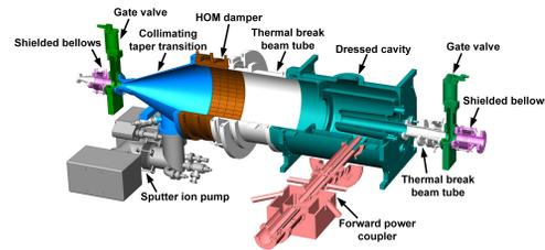
Figure 1: The 166 MHz cavity string.
