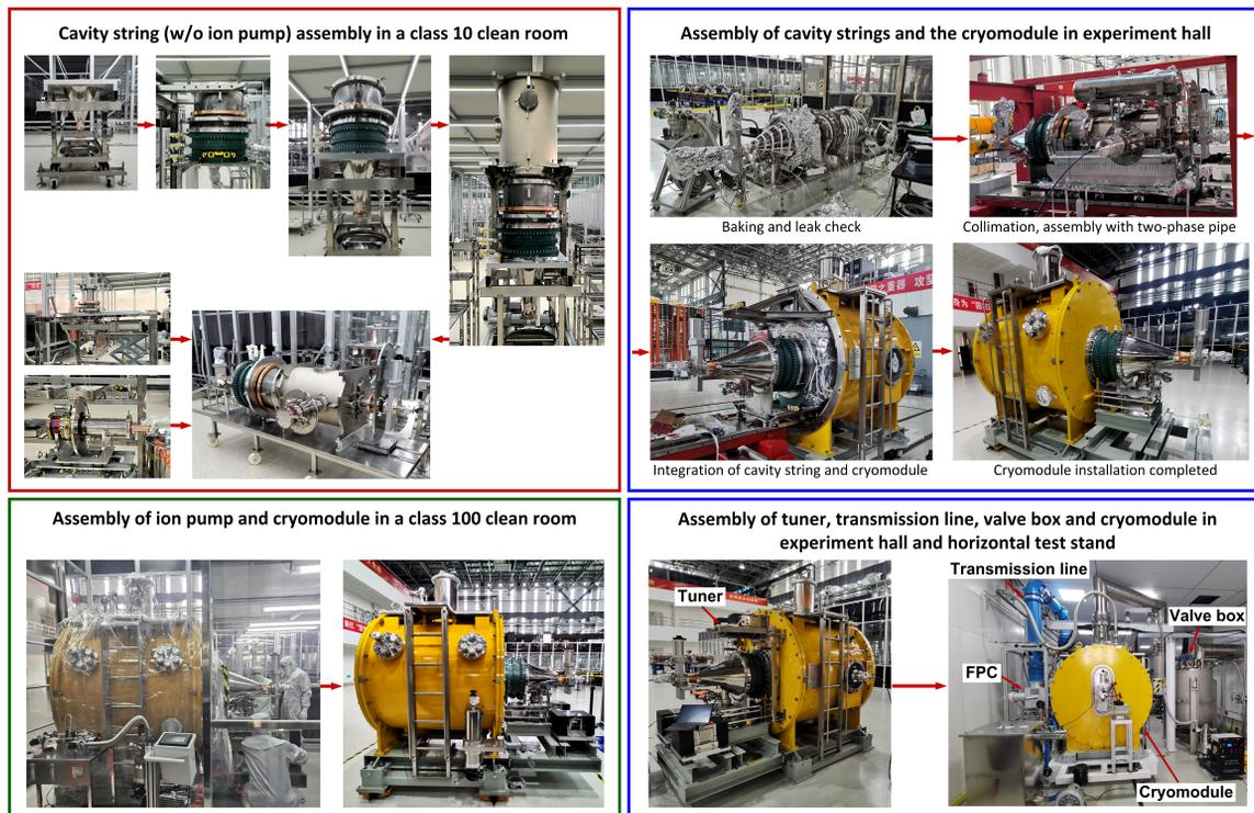
Figure 6: Assembly of the 166 MHz cavity string and the cryomodule.
