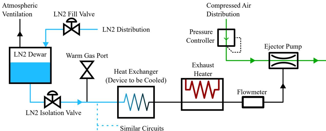
Figure 2: A diagram of the VACCS system. Liquid nitrogen is represented with blue lines, gaseous nitrogen with black lines, and air with green lines.
