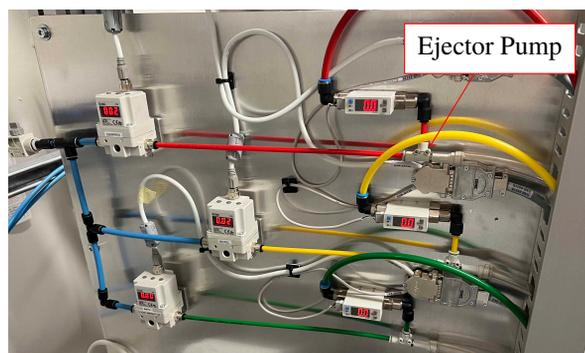
Figure 4: The pneumatic control system for the three zones on VMXm. Sample gripper zone (red tubing) on top, the sample hotel zone (yellow tubing) in the middle, and the anti-contaminator zone (green tubing) at the bottom.
