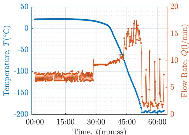
Figure 5: Cool down of the sample gripper. The left axis depicts the temperature of the gripper, while the right axis depicts the flow rate of GN2.
