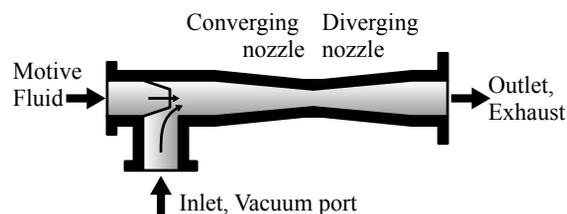
Figure 1: An illustration of an ejector pump (Figure based on a diagram from the product sheet in [2]).
