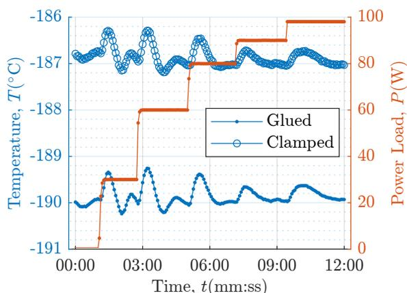
Figure 9: Power load variation on the test rig. The glued PT100 is depicted with pointed markers and the clamped PT100 circle markers.
