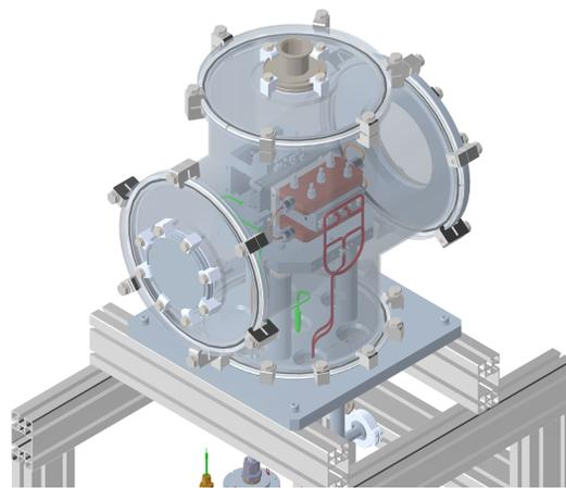
Figure 7: A CAD model of the monochromator test rig for validating the application of the VACCS system.
