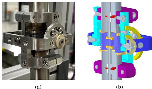
Figure 3: Joint of a flexible LN2 distribution line. (a) a picture of a joint on VMXm, (b) a section view of the CAD model.
