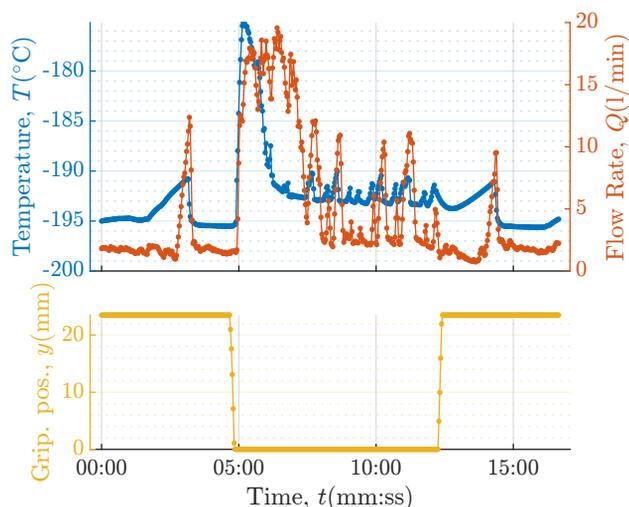
Figure 6: Cooling performance of the sample gripper. The upper plot depicts sample gripper and flow rate of GN2, on the left and right axis respectively, while the lower plot depicts the vertical position of the sample gripper.
