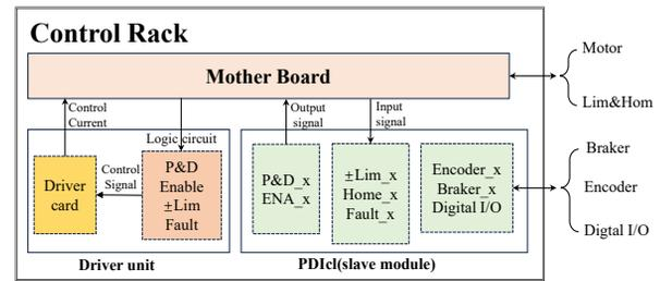
Figure 4: The way of processing of signal inside the control rack.
