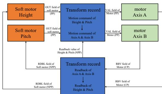
Figure 5: The control logic of whit beam mirror
