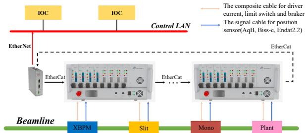
Figure 1: The overall hardware architecture of HEPS MCS.
