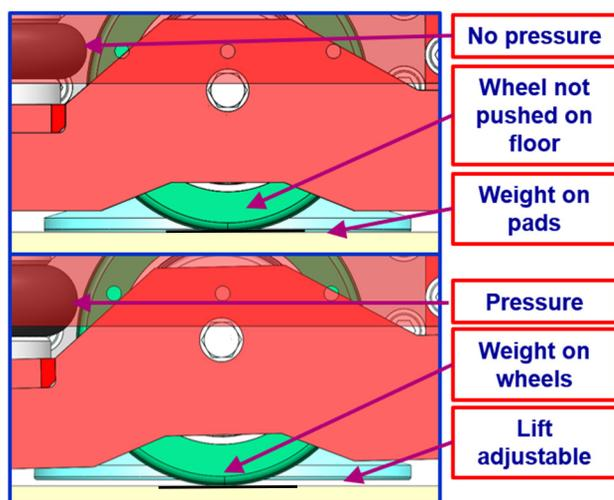
Figure 9: Main wheels in retracted position (top figure) and in contact with the floor (bottom figure).
