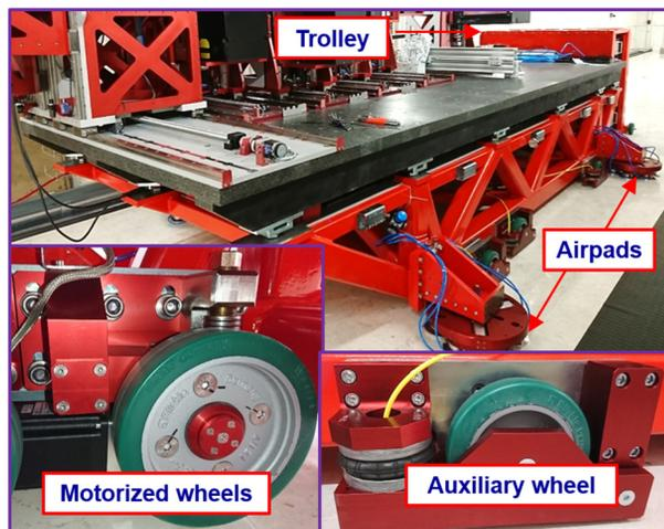
Figure 7: Detector girder on airpads. Details of motorized wheels and auxiliary wheels.
