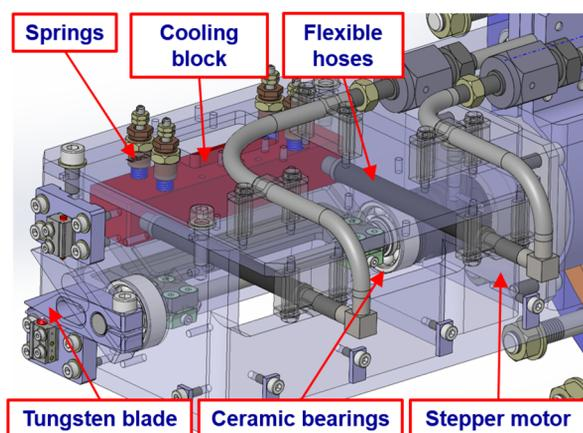
Figure 1: Design of the in-vacuum cooled fast shutter.
