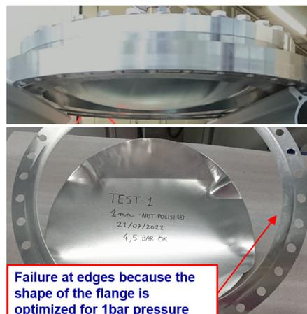
Figure 5: Aluminium window during water pressure test.
