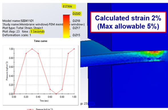
Figure 4: Strain calculation of the membrane showing a deformation of 2 % (5% is the failure deformation obtained during the collapsing tests).
