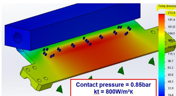
Figure 2: Temperature rise of the tungsten blade relative to the water temperature.
