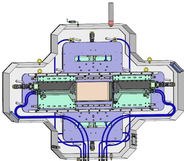
Figure 6: Picture and layout of the quinary slits inside the nitrogen box. A 25 μm Kapton window has been installed for 7 months now without failure.
