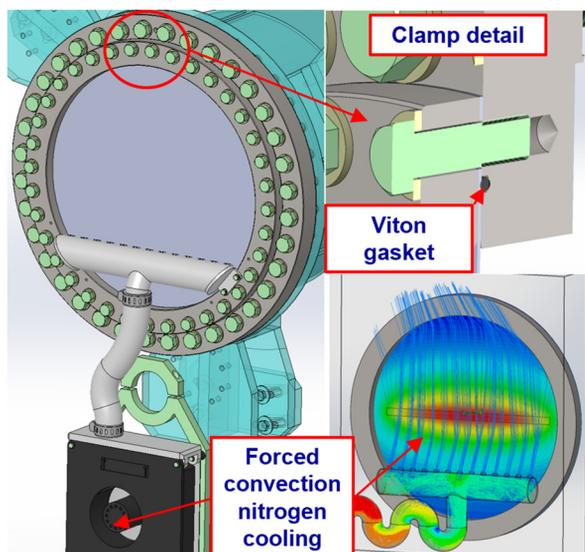
Figure 3: Design and thermal simulation of the membrane.
