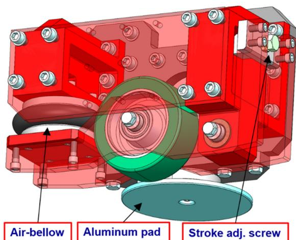
Figure 8: Main wheels to replace of the airpads.
