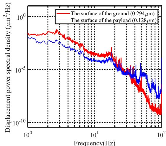
Figure 2: The comparison of the displacement power spectral density in the direction of gravity when the active vibration control is on.
