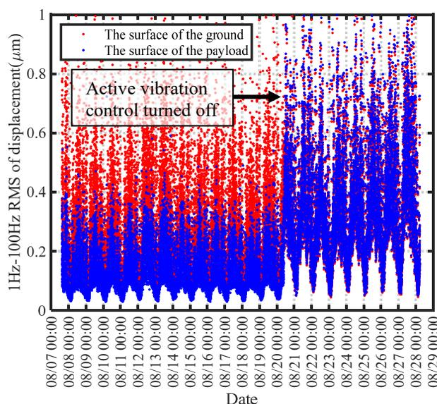
Figure 3: Long-term test results of displacement RMS.
