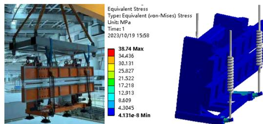
Figure 11: Lifting method and stress FEA results.
