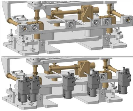
Figure 4: UAP Platform in manual and motorized versions.
