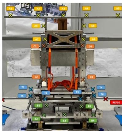
Figure 3: UAP Platform during test with a dummy collimator. Each cross represents a measurement target installed during the tests.
