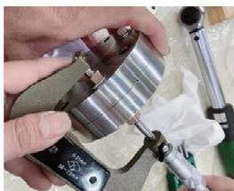
Figure 9: Length measurement.
