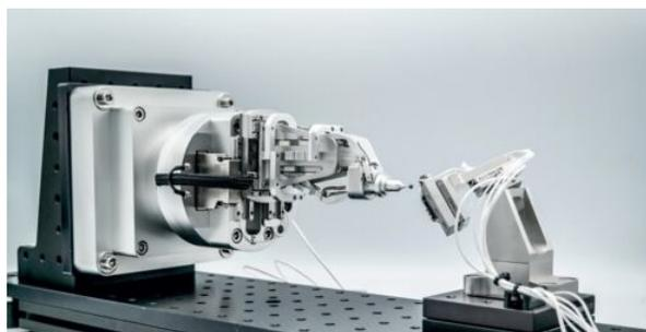
Figure 3: The calibration setup involves rotating a calibration sample, a sapphire sphere ( $D=2\text{mm}$ ) around each of the rotation axes individually and measuring the runout in three dimensions (XYZ). This is negatively fed back into smargopolo as a translation.
