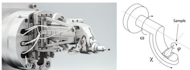
Figure 1: SmarGon with a representation of the rotations  $\omega$ :  $[-\infty, +\infty]$ ,  $\chi$ :  $[0, 90^\circ]$ ,  $\phi$ :  $[-\infty, +\infty]$ .
