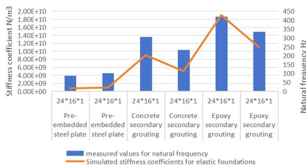
Figure 6: Same foundation dimensions and different connection methods.
