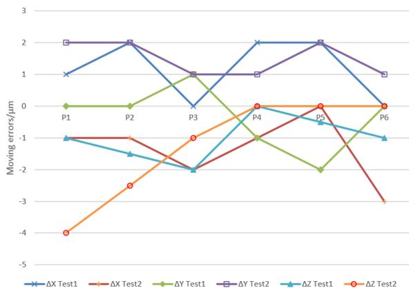
Figure 14: Motion precision test result.
