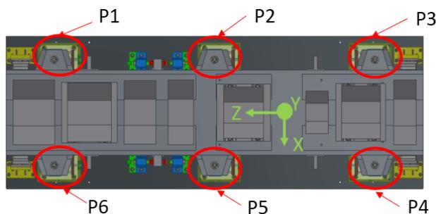
Figure 13: Schematic diagram of measuring point.
