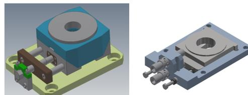
(a) Girder body adjustment (b) Magnet adjustment
